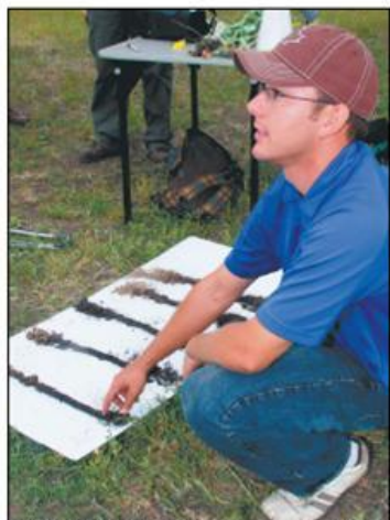
Once the Veris has identified distinct soil variations in a field, Justin Cleaver takes core samples that are used to ground truth the Veris data. (W/P photo by Ron Lyensing)
