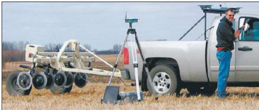
Since the spring of 2008, CropPro mapping consultant Brad Dunnington has logged 40,000 acres, simultaneously mapping EC and topography with this Veris 3100 linked to an AutoFarm RTK GPS unit. (Photo courtesy of Cory Willness/CropPro Consulting)
