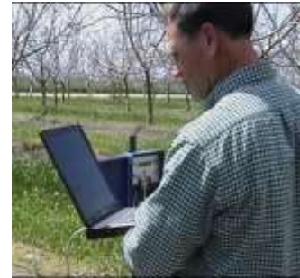
Manual Data Download using a Laptop
