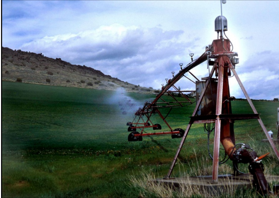
Figure 12-17: Center-pivot Sprinkler Irrigation Systems Using a Well as a Source of Water, Idaho
