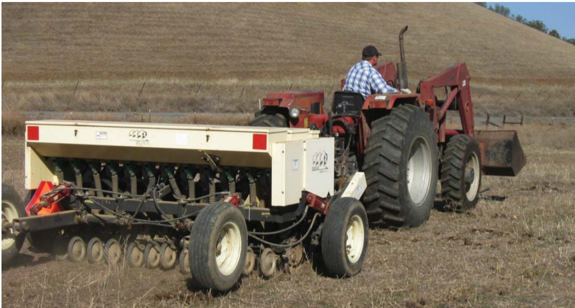
Photo: (above) Native seed drills are the ideal tool for large planting sites (5+ acres). Typical models can plant in a light stubble layer, have depth controls for optimal seed placement, and have separate seed boxes for different sizes of seed. Such drills need an experienced operator and careful calibration. (Photo: Jessa Guisse, Xerces Society).
